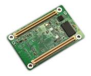
The A5S receiving card is connected to the Hub board through the card slot. Meanwhile, the Hub board which plays the role of transit is also connected to the module, power supply and data cable.
