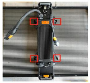
Step 2, Place the power supply horizontally and open the cover.
