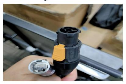
LR series network cables and power cables are connected by aviation heads, as above: Note: The connecting cables between the cabinets should pass through the cabinets as much as possible. If the connection method changed, please set the same connection method in the software settings. Please refer to the software for more details.
