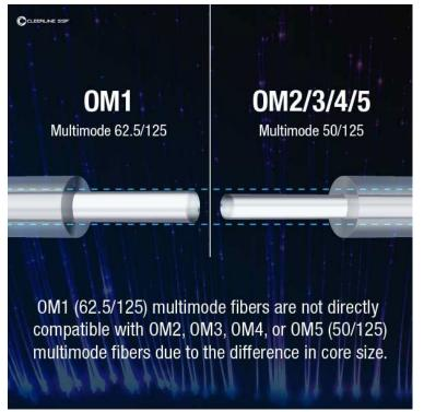
Importantly, OM1's 62.5 µm core size means that it is not compatible with other grades of multimode and cannot accept the same connectors. Since OM1 and OM2 can both have orange outer jackets (per TIA/EIA standards), always check the print legend on the cable to ensure you are using the correct connectors.
