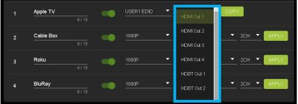
**Input Settings Signal** - The Signal Indicator on the HDMI INPUTS shows the current state of the connection HDMI source. Green means the HDMI source is detected, red means that the source is not detected. If red verify that source is powered on and that the HDMI cable is
