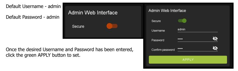
With the Admin Web Interface enabled, the only menu that will be accessible using the WebUI will be the Matrix tab. The rest of the settings will require the Admin log in to access.
